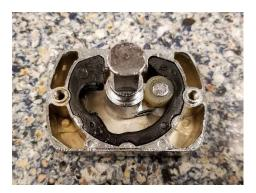
Next, pull out the internal components and set them aside. Place all new pieces back into the housing in reverse order, being sure to face the parts in the same direction as before. General purpose grease is recommended to be placed on the rubber "C" bumper to ensure long-lasting service.
