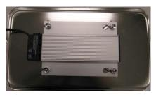
Figure 2. Electric Heating Element, Mounted Alignment
