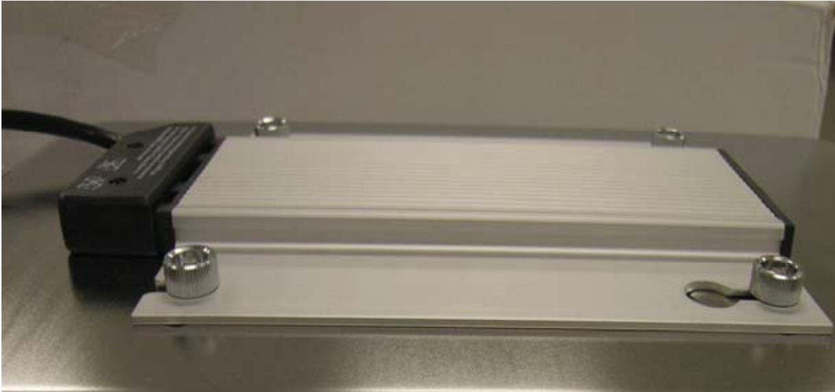
Again, the heating element must be flush with the water pan – you should not see any gaps between the element and the pan. If there is a gap, ensure the bolts are tight. If a gap still remains after you have tightened the bolts, you may have a warped water pan.
