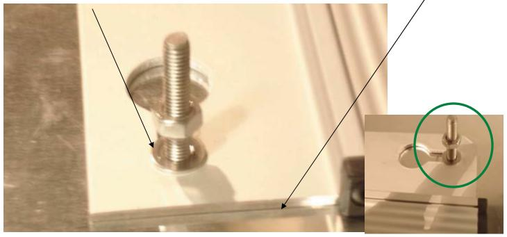
Tighten the nut to the base of the Electric Heating Element. Continue until all four nuts are flush with the Heating Element.
