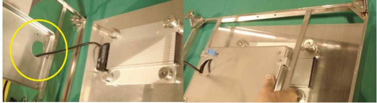
Feed the cord from the Electric Heating Element into the cord fastener and push until it is secure in the track. While supporting the underside of the base, begin replacing all the thumb screws. Replace all four screws.
