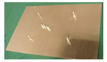
Loosen the nut so it remains approximately 1/4" above the metal base and lift the washers on all four screws.
