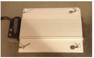
Replace the four long, thin cylinders onto the screws. Then replace four round, thick cylinders.
