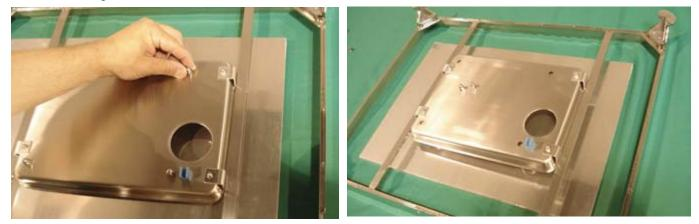
Remove the Carving Station frame and set aside. Remove the four (4) round, thick cylinders and set aside.
