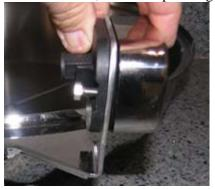
6. Remember, with the server being flipped, insert the right axle, (marked with a "R" on the black axle leg) to the left side. Insert the Left axle (marked with a "L" on the black axle leg) on the right side of the server. Use the wrench to tighten the screws in place. Replace the server cover.
